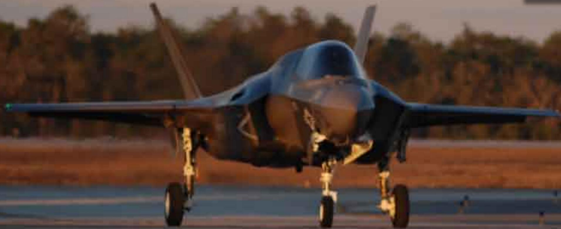
MOVING 360 DEGREES AROUND AN F-35 ONE WORD COMES TO MIND "SEAMLESS" POSSESSING THE RADAR SIGNATURE OF A GOLF BALL, VIRTUALLY THE ONLY SEAM TO BE FOUND IS ALONG THE ENGINE'S REAR EDGE.
