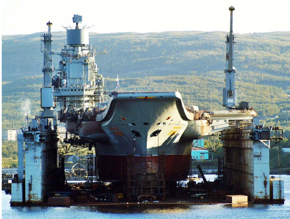
Figure 20. Admiral Kuznetsov inside the PD-50 floating drydock (From Pieter Inpyn, 2010)
