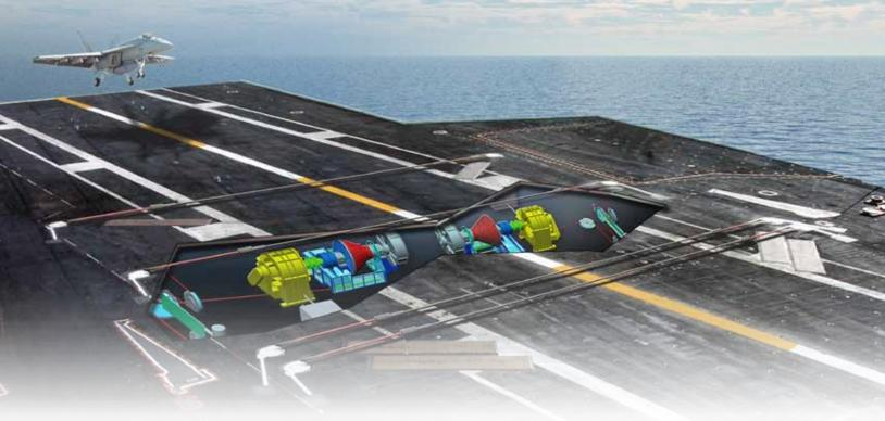
The General Atomics AAG Team has assembled a full-scale shipboard representative system that is undergoing testing at the NAVAIR-Lakehurst, N.J. AAG will be installed on the CVN 78 Ford-class aircraft carrier. The system will also be installed on CVN 68-class aircraft carriers during refueling overhaul to replace the current Mk-7 arresting gear system.
