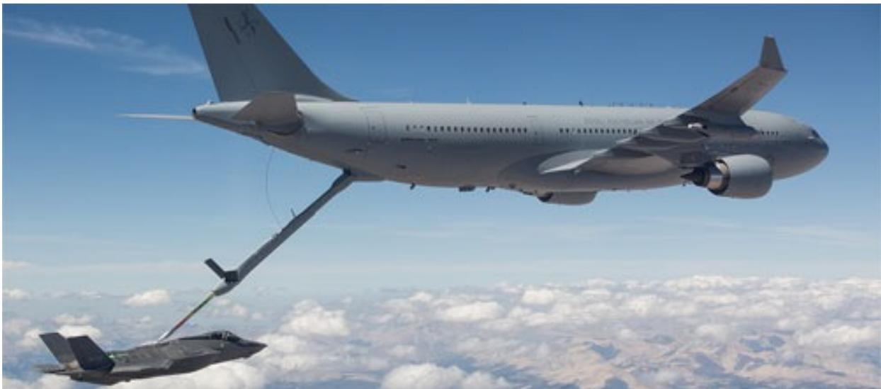
The Aussies have kept one KC-30A on station during the operations. It has had an outstanding 95% reliability rate, and has been rapidly certified to do tanking operations on a variety of coalition aircraft, including Canadian ones.
