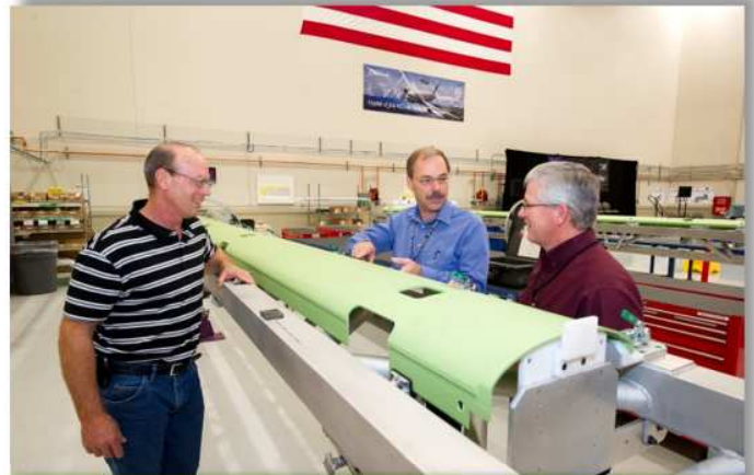
Tanker teammates Chris Johnson, Jim Prideaux and David Dean examine the first KC-46 boom skins that will undergo assembly.
